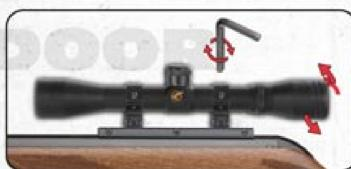
5 Before tightening the screws in the upper half of rings, align (rotate) the vertical and horizontal post axes of the reticle with the vertical and horizontal (bore) axes of the airgun. You can tighten all ring mounts screws using a non permanent thread lock.
